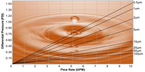
Flow multiply differential pressure by fluid visco
